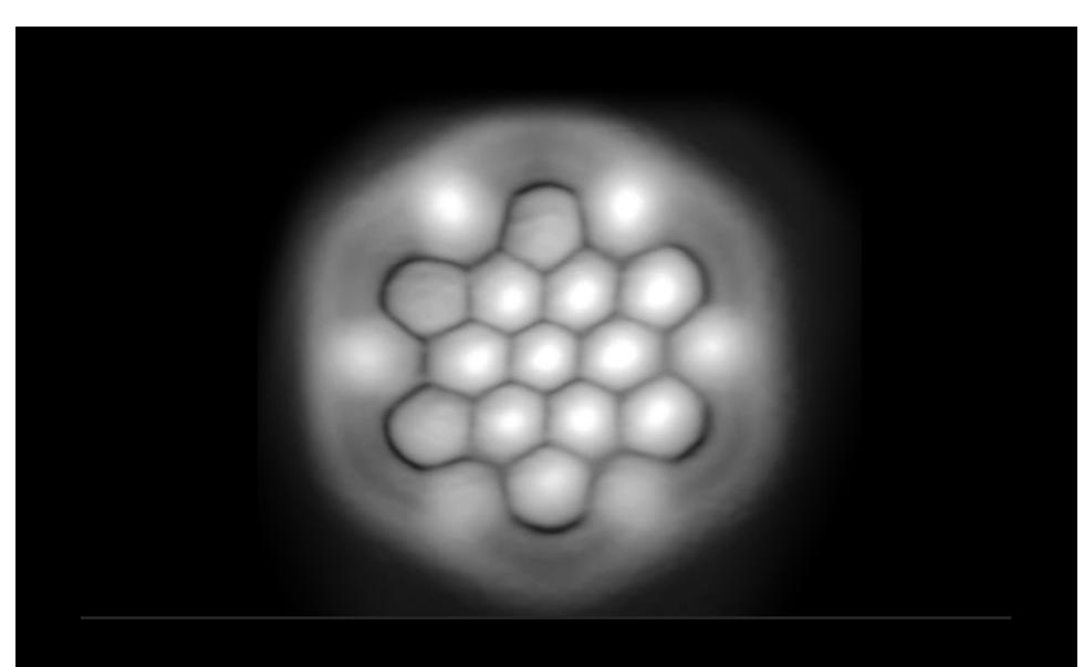
Created by IBM scientists in Zurich, Switzerland, using noncontact atomic force microscopy, the image shows the varying electron concentration around a molecule of nanographene.
